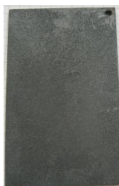
Figure 3. Substrate surface surface after phosphatizing coating
