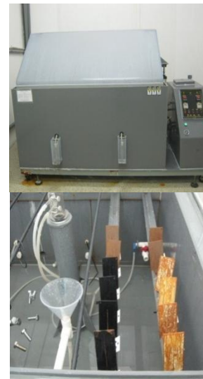
Figure 1. Salt chamber front panel and position of tested samples during the test
