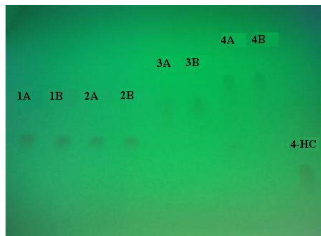
Figure 2. TLC plate developed with mobile phase 6 , under the UV light on 254 nm for the compounds 1 – 4 (raw substances ( A ) and after purification process ( B ); 4-HC at the end)
